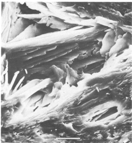
Figure 7 SEM micrograph of the fractured surface of a heavily etched (49% HF for 30 sec) AISiPYO glass crystallized using a heat treatment of only 1673 K for 14.4 \times 10^3 sec. (Bar = 10.0 \times 10^{-6} m).
